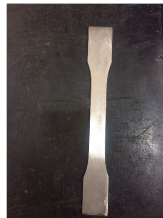
Figure 2 Tensile Test Specimen for the welded assembly
