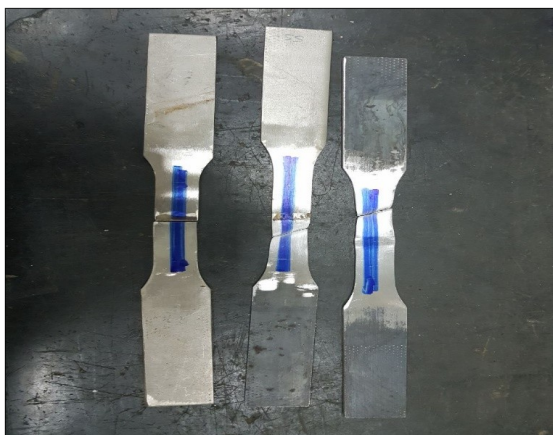
Figure 6 Fractured Weldments of MS-SS plates
