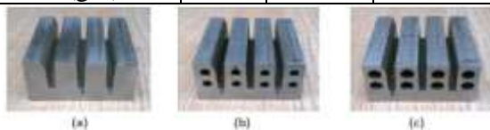
Figure 3: Schematic view of the fin arrays (a) Fin without perforation, (b) Fin with two perforations of 5mm, (c) Fin with two perforations of 7mm.
