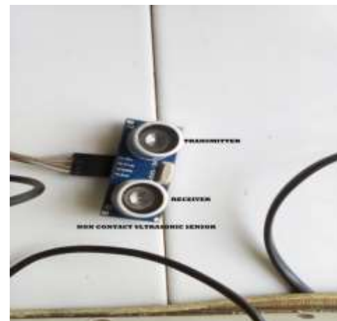
Fig. 6: shows the Transmitter (T: up) and Receiver (R: down) of the Ultrasonic sensor
