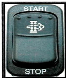
Fig 4 : Forced regen Switch in Dashboard
