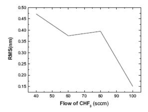
**Figure 1:** Effect of the flow rate of CHF<sub>3</sub> on the surface roughness of the etched surface.
