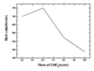
**Figure 2**: Etch rate of silicon carbide as a function of the CHF<sub>3</sub> flow rate.
