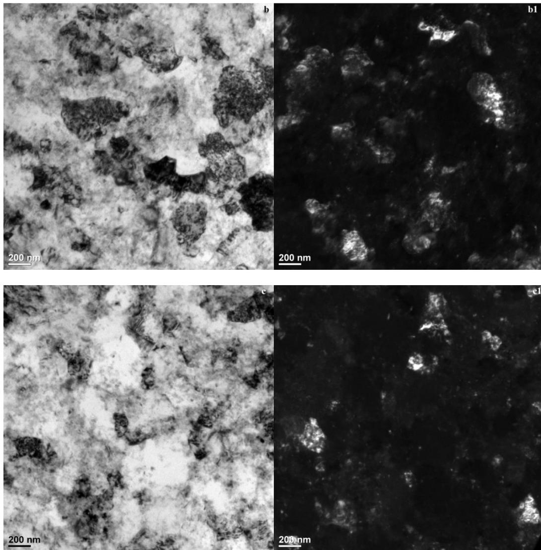
**Fig.3:** Bright field and dark field TEM images of (a) and (a1) Al-5vol.% Al<sub>2</sub>O<sub>3</sub> nanocomposite powder produced by HEMM; (b) and (b1) Al-5vol.% Al<sub>2</sub>O<sub>3</sub> nanocomposite disk produced by powder compact forging; (c) and (c1) Al-5vol.% Al<sub>2</sub>O<sub>3</sub> nanocomposite rod produced by powder compact extrusion.
