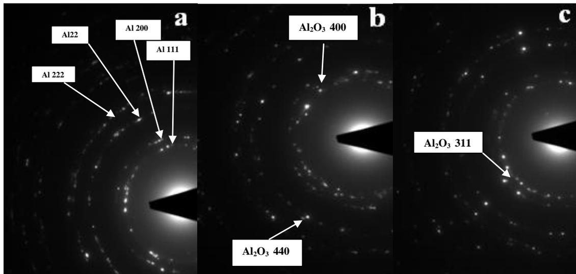
**Fig.4:** Selected area electron diffraction patterns of (a) Al-5vol.%Al<sub>2</sub>O<sub>3</sub> nanocomposite powder produced by HEMM, corresponding (a) and (a1) in Fig. 3; (b) Al-5vol.%Al<sub>2</sub>O<sub>3</sub> nanocomposite disk produced by powder compact forging, corresponding (b) and (b) in Fig. 3; (c) Al-5vol.%Al<sub>2</sub>O<sub>3</sub> nanocomposite rod produced by powder compact extrusion, corresponding (c) and (c1) in Fig. 3.
