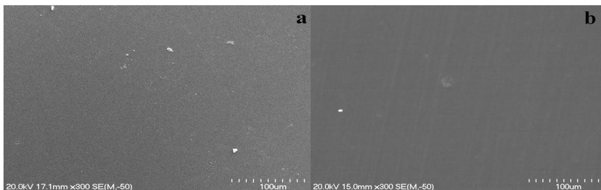
**Fig. 5:** SEM micrographs of the central part of cross sections of (a) Al-5vol.%Al<sub>2</sub>O<sub>3</sub> nanocomposite disk produced by powder compact forging; and (b) Al-5vol.%Al<sub>2</sub>O<sub>3</sub> nanocomposite rod produced by powder compact extrusion.
