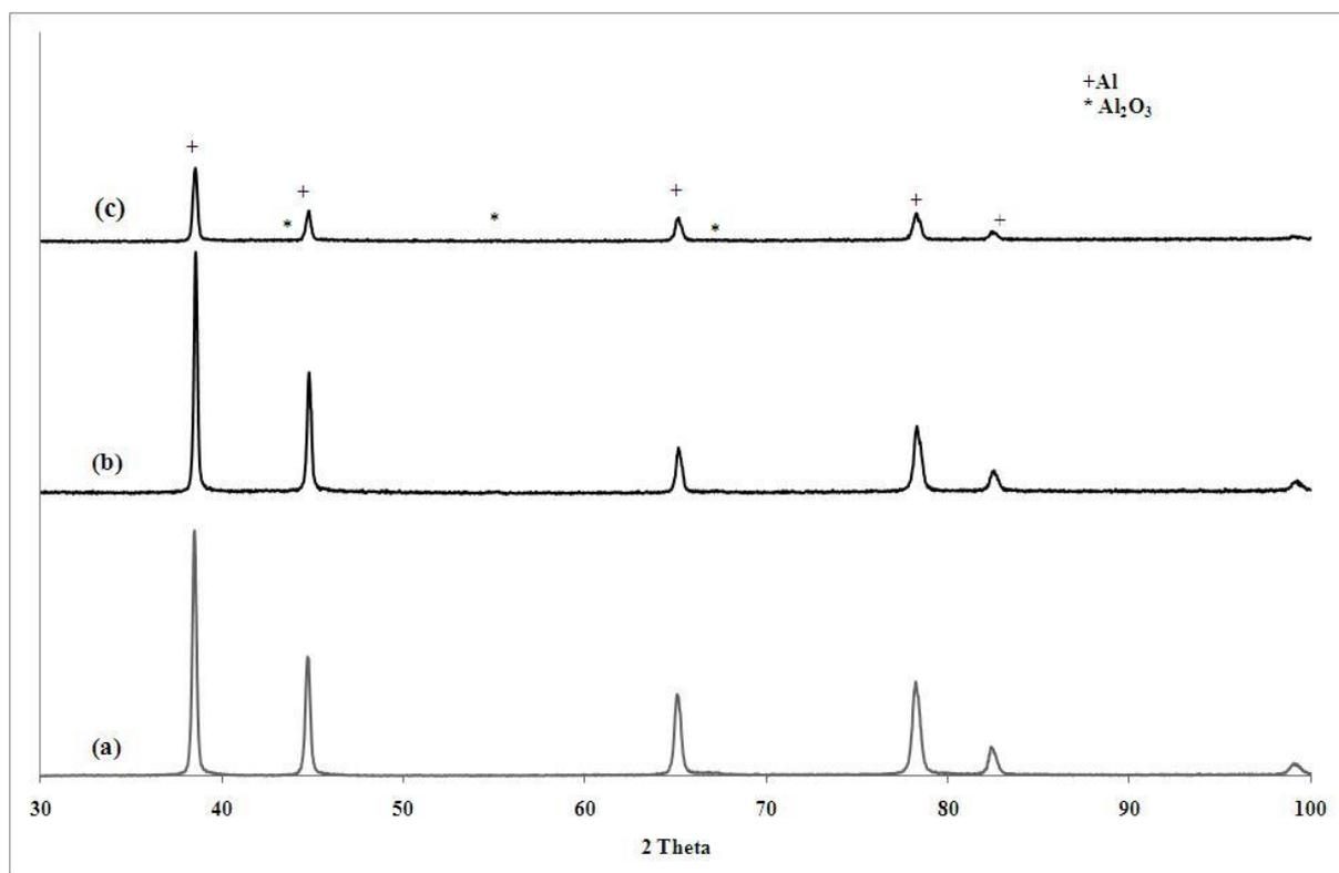
**Fig.1:** XRD patterns of (a)Al-5vol.-%Al<sub>2</sub>O<sub>3</sub> nanocomposite powder produced by HEMM; (b) Al-5vol.-%Al<sub>2</sub>O<sub>3</sub> nanocomposite disk produced by powder compact forging; (c) Al-5vol.-%Al<sub>2</sub>O<sub>3</sub> nanocomposite rod produced by powder compact extrusion.
