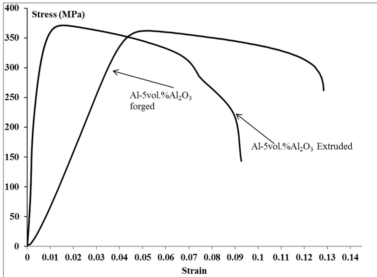
**Fig. 6:** Tensile engineering stress-strain curves of specimens Al-5vol. %Al<sub>2</sub>O<sub>3</sub> nanocomposite specimens cut from Al-5vol.%Al<sub>2</sub>O<sub>3</sub> nanocomposite disk produced by powder compact forging and Al-5vol.%Al<sub>2</sub>O<sub>3</sub> nanocomposite rod produced by powder compact extrusion, respectively.
