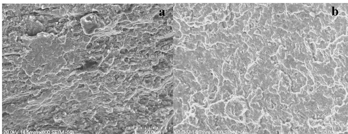
**Fig. 8:** SEM micrographs of the fracture surfaces of the tensile tested specimens cut from Al-5vol.% Al<sub>2</sub>O<sub>3</sub> nanocomposite samples produced by (a) powder compact forging and (b) powder compact extrusion, respectively.
