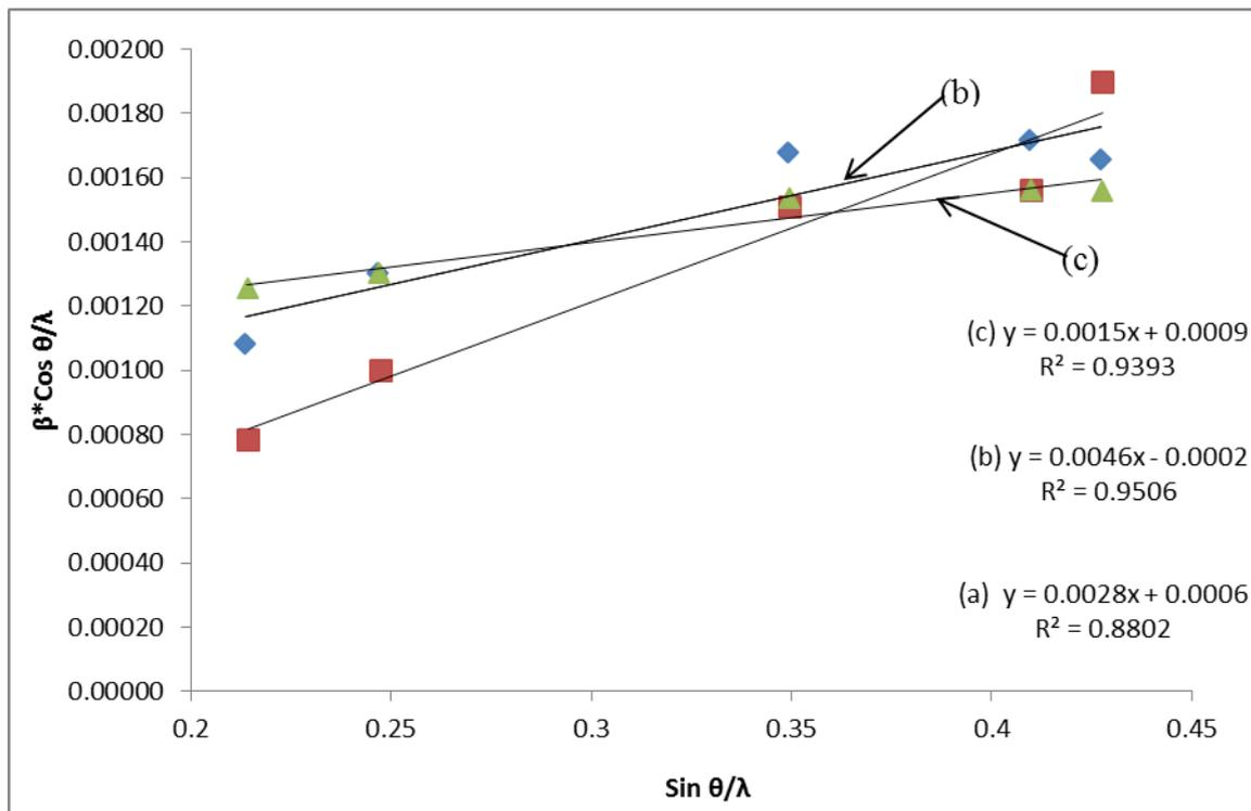
**Fig.2:**  $\beta \cdot \cos \theta / \lambda$  vs  $\sin \theta / \lambda$  plots: (a) Al-5vol.%  $\text{Al}_2\text{O}_3$  nanocomposite powder produced by HEMM; (b) Al-5vol.%  $\text{Al}_2\text{O}_3$  nanocomposite disk produced by powder compact forging; (c) Al-5vol.%  $\text{Al}_2\text{O}_3$  nanocomposite rod produced by powder compact extrusion.
