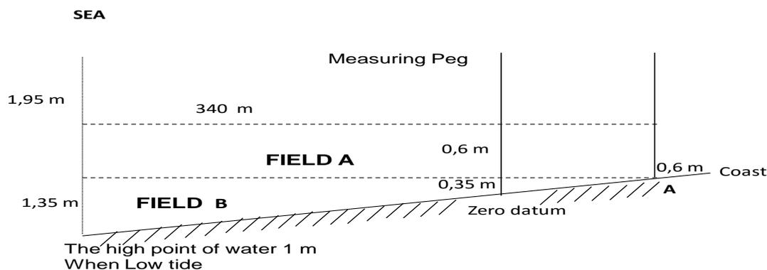
Figure 4. Field construction measurements at sea
