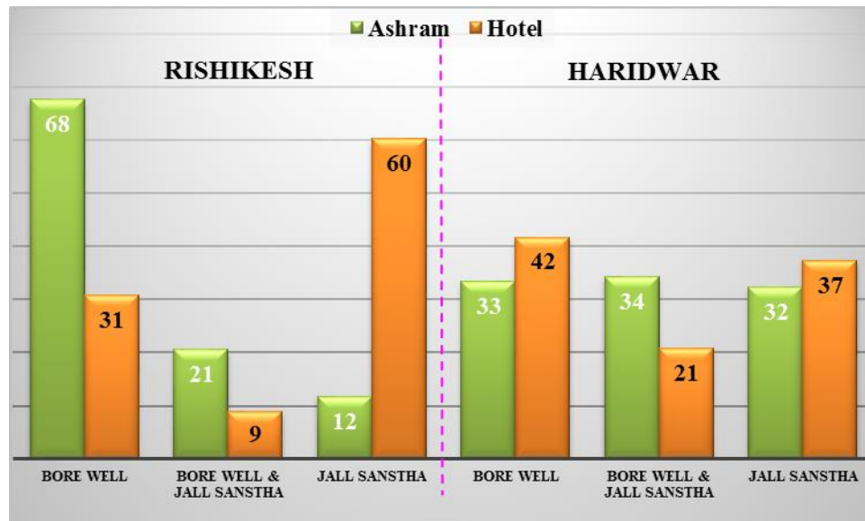
Figure 4: Fresh water sources and various utilization in Rishikesh and Haridwar.
