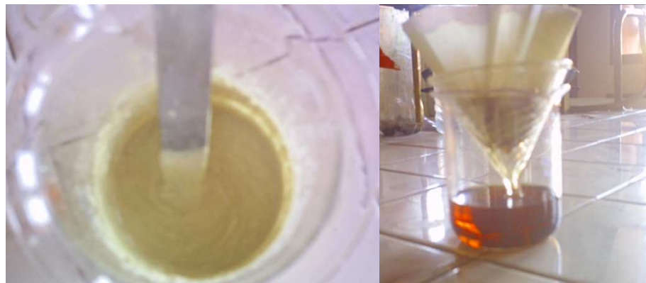
Figure 10: ferric Sulphate before the solubilizations (on the left) and after solubilizations and filtration (on the right)
