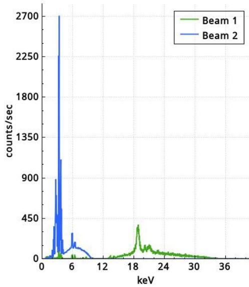
**Figure 1: X-ray spectrum of a tea sample (green tea) by HHXRF**
