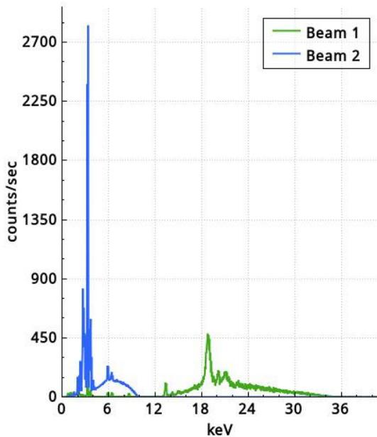
**Figure 2: X-ray spectrum of a tea sample (black tea) by HHXRF**
