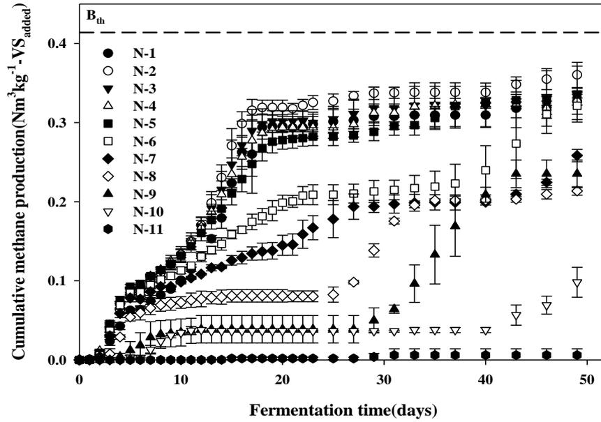
Fig. 3. Cumulative methane production curves influenced with increased ammonia concentrations in anaerobic batch reactors (Vertical bars mean standard deviations,  $B_{th}$  is theoretical methane potential of cellulose, N-1, N-2, N-3, N-4, N-5, N-6, N-7, N-8, N-9, N-10, and N-11 are 1,000, 2,000, 3,000, 4,000, 5,000, 6,000, 7,000, 8,000, 9,000, 10,000, and 13,000 mg-total ammonia nitrogen/L, respectively).
