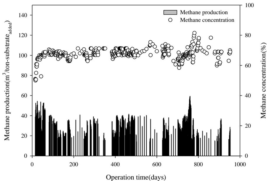
Fig. 1. Methane productions (m<sup>3</sup>/ton-substrate<sub>added</sub>) and methane concentrations (%) changes monitored from an inoculum-donor anaerobic digester for a period of 1,000 days. The anaerobic digester is a 190 m<sup>3</sup> farm-scale digester (Anseong, South Korea) operated at a temperature of 38°C and a hydraulic retention time of 30 days using pig slurry.
