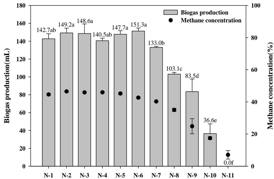
Fig. 2. Biogas productions and methane concentrations influenced with increased ammonia concentrations in anaerobic batch reactors (Means with different character differ significantly ( $p < 0.05$ ) (N-1, N-2, N-3, N-4, N-5, N-6, N-7, N-8, N-9, N-10, and N-11 are 1,000, 2,000, 3,000, 4,000, 5,000, 6,000, 7,000, 8,000, 9,000, 10,000, and 13,000 mg-total ammonia nitrogen/L in the reactors, respectively).
